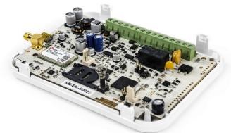
ET082 is a universal GSM/GPRS, PSTN, LAN gateway/communicator, which expands any PSTN intrusion alarm panels functionality and adds communication channels. The panel can then communicate with alarm receiving centers and directly to home owner, as well.
